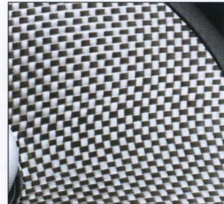
Membrane DFS ® Cone Dual Fiberglass Structure
