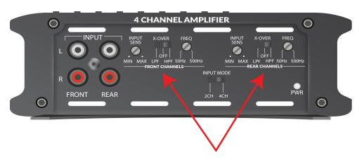
**Tuning/Configuration knobs & switches:**
