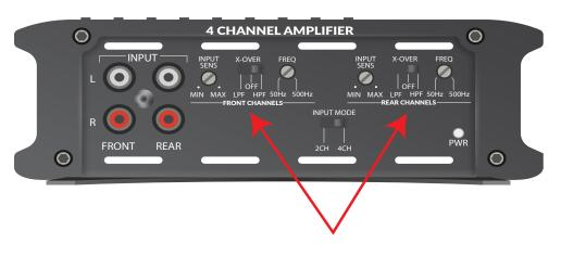
**Tuning/Configuration knobs & switches:**
