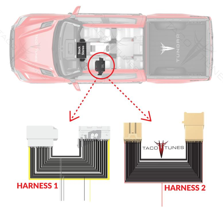
Harness 1 & 2 plug directly into the factory JBL amplifier & the factory wiring of your Tundra
