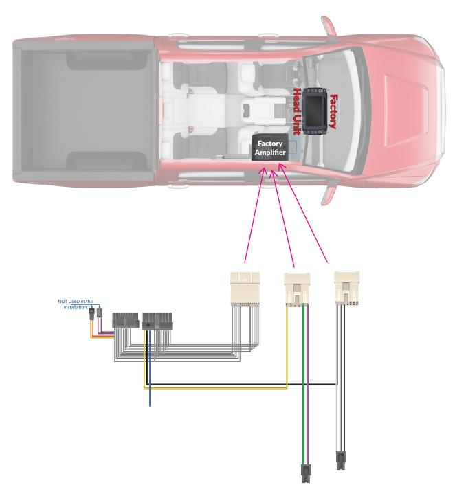
Harness plugs directly into your factory wiring under the passenger seat.
