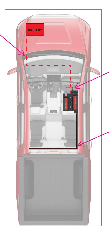
Connect to factory wiring under seat, & to TXD Amplifiers:
