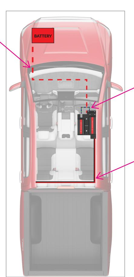
Connect to factory wiring under seat, & to Amplifiers:
