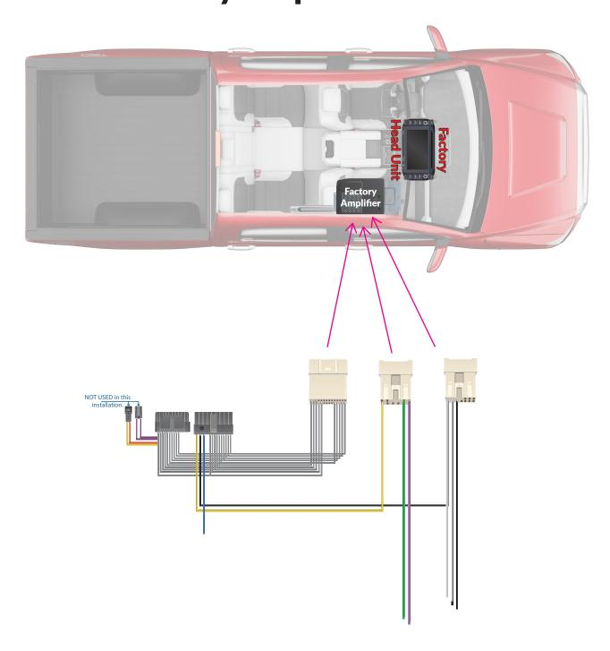
Harness plugs directly into your factory wiring under the passenger seat.
